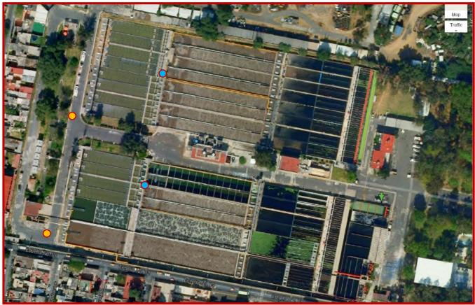
Installed capacity (I/s): 3000 Treated flow (I/s): 2300 Process: Activated sludge
