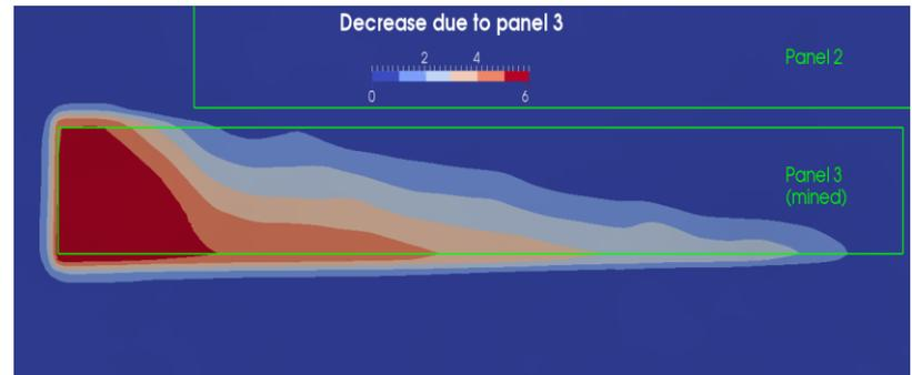
Gas release pattern from Wambo seam
