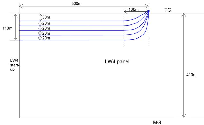
Plan view of roof lateral holes
