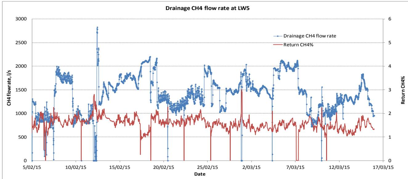
LW5 drainage CH4 flow rate to 15/03/2015 (retreat of 398 m)
