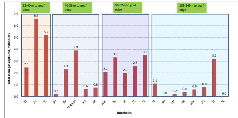
Effect of well location on drainage preformation
