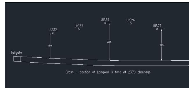
Roof lateral holes placed at 15-22m above mining seam
