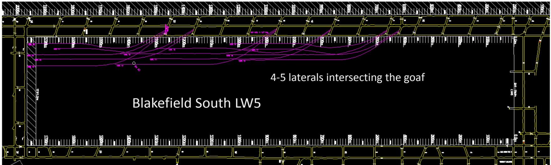
LW5 goaf gas drainage roof lateral holes
