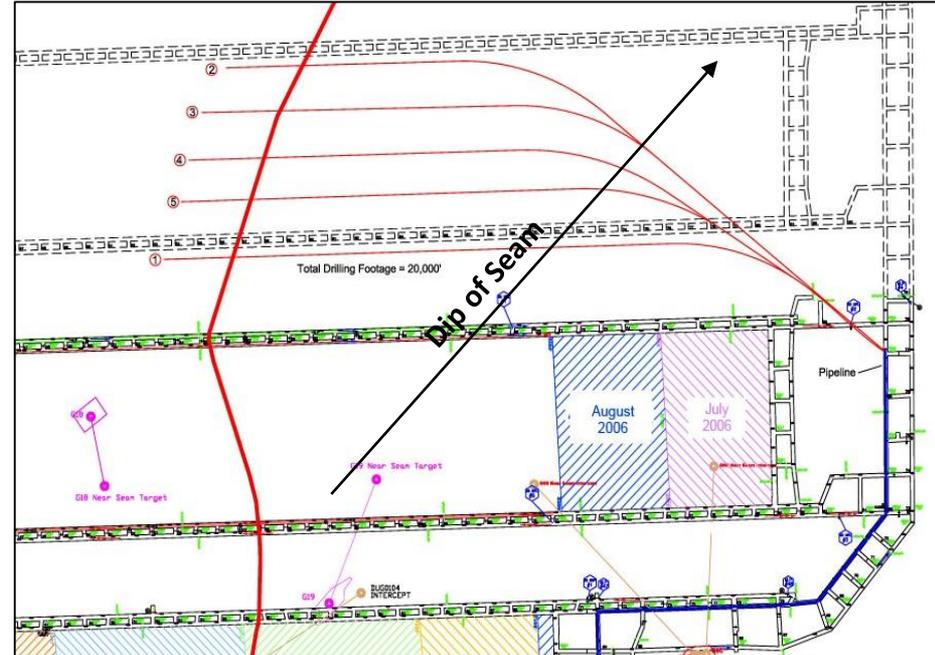
■ Boreholes Placed Up-Dip to Efficiently Manage Water Accumulation
