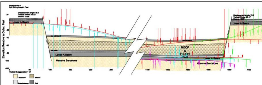
■ Borehole Placement to Consider Geologic Structure
