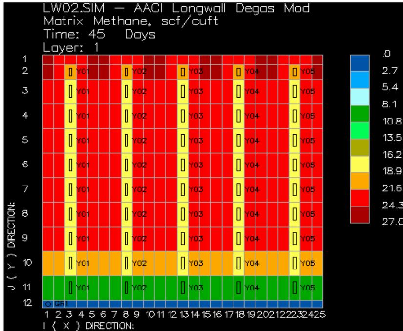
$GC_I = 15 \text{ m}^3/\text{t}$ , Spacing 20 m
