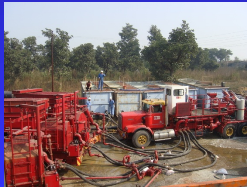
Hydro-frac unit at 3 rd Well
