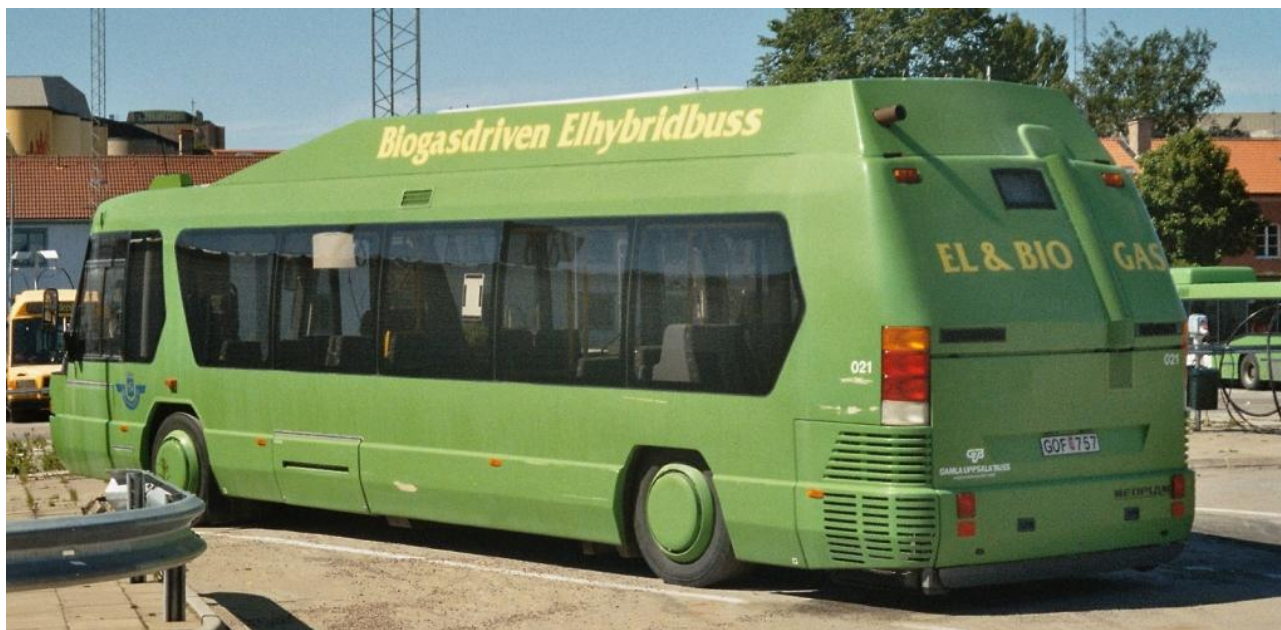
Figure 2.10. Biogas (CBG) hybrid bus in Uppsala, Sweden, using biogas produced at sewage treatment plant. City buses are the most important short term applications of traffic biogas.
