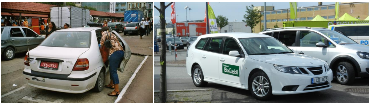
Figure 2.12 Methane/ethanol/gasoline multifuel cars: a) Fiat Siena Tetrafuel (E100) in Manaus, Brazil. b) Saab Trifuel (E85) in Gothenburg, Sweden.
