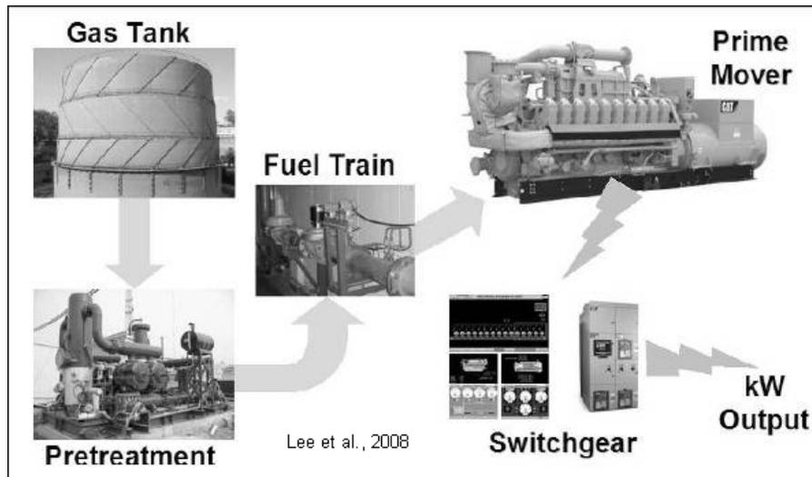
Figure 5-1: Stages of the CMM to Power Generation Process
