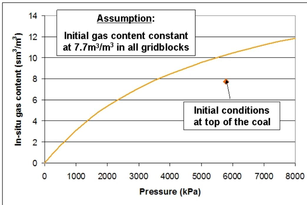
Figure 4-11: Sorption Isotherm for Coal Seam 13-1
