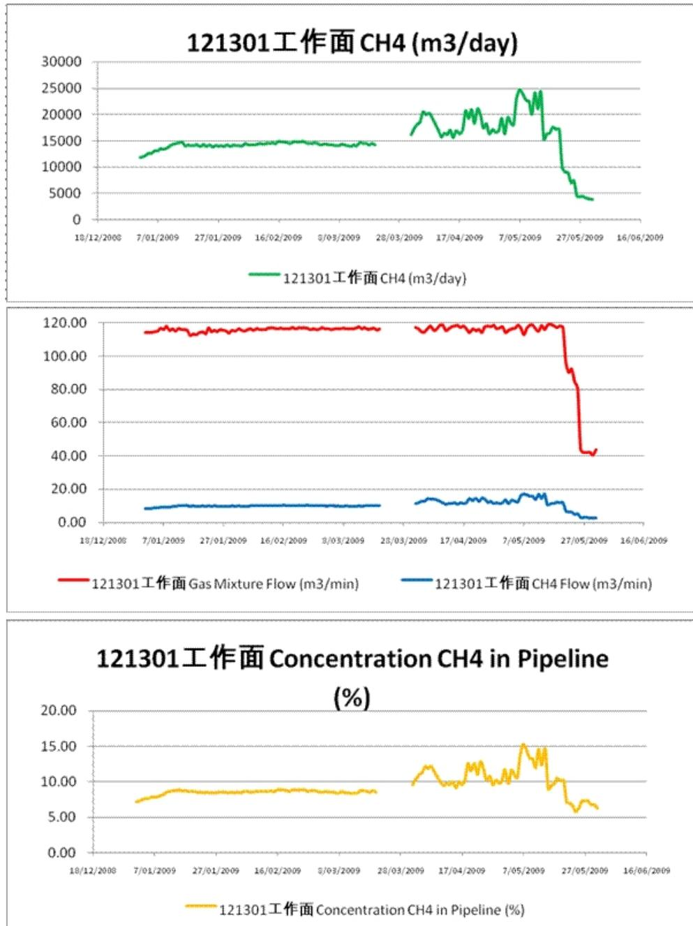
**Figure 4-8: Detailed Hourly Methane Flow Rate and Concentration**
