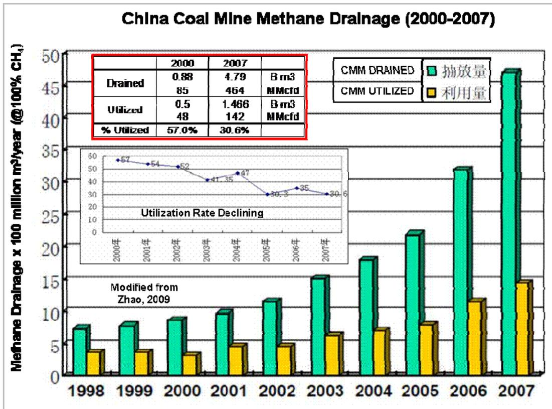
Figure 1-3: CMM Drainage and Utilization in China
