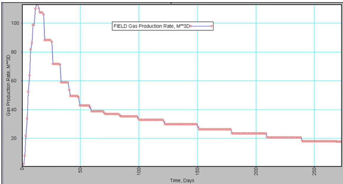
**Figure 4-14: Simulated Methane Production from a Horizontal In-Seam Borehole at Liuzhuang**
