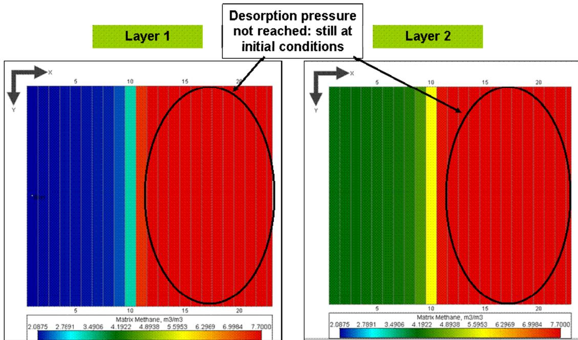
**Figure 4-13: Simulated Reduction in Gas Content**
