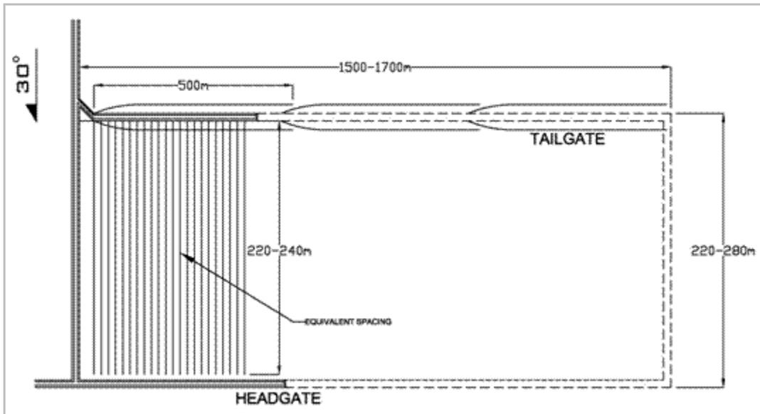
Figure 4-15: Alternative Drainage Drilling Scenario No.1
