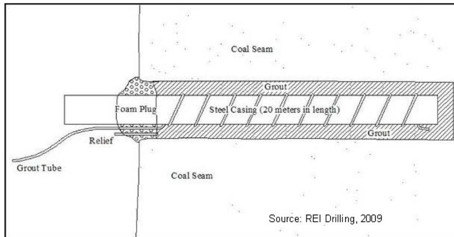
Figure 6-8: Preliminary Design for Improved Borehole Completion
