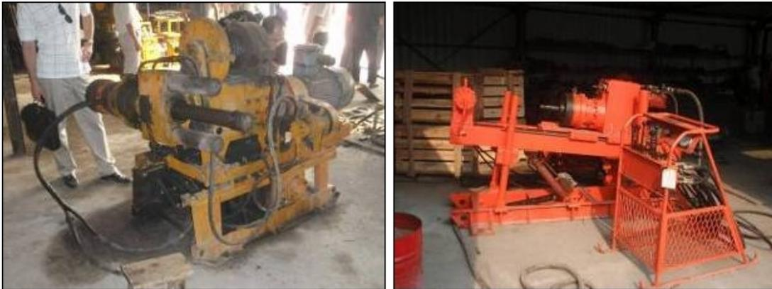
**Figure 4-3: Short Horizontal Borehole Drills Used at Liuzhuang Mine**
