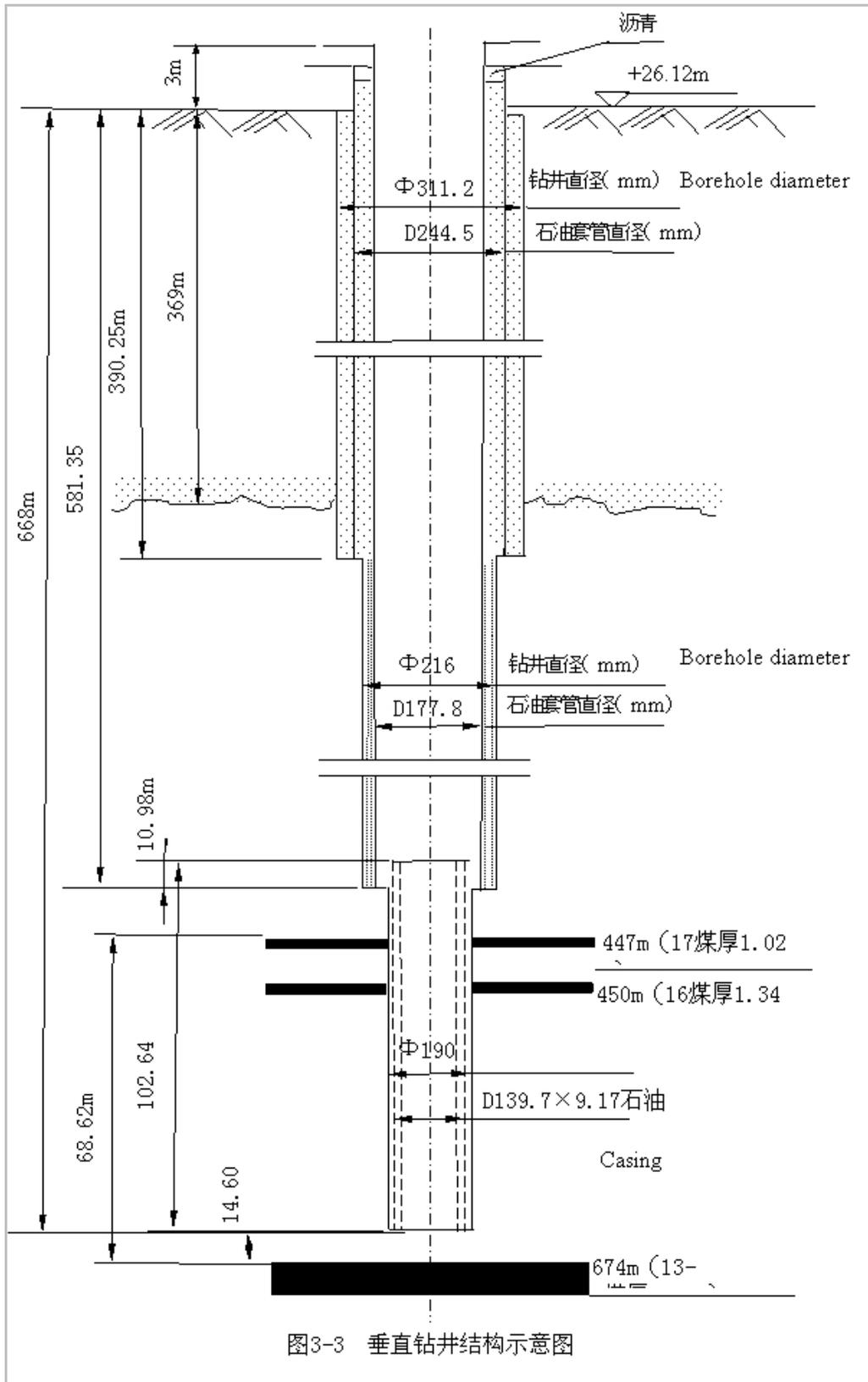
Figure 4-25: Gob Well Casing String Design at Liuzhuang mine
