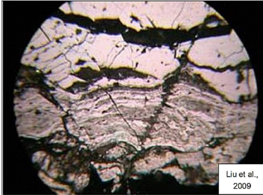
**Figure 1-8: Photomicrograph (300x) of a Coal Sample in the Huainan Coal Field**
