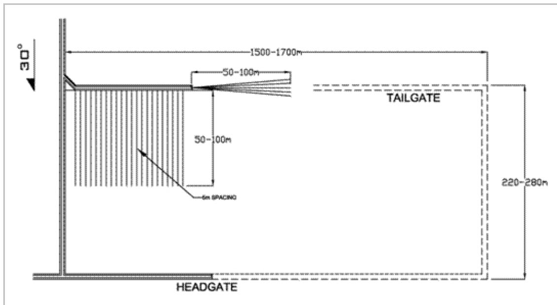
Figure 4-9: Schematic of Current CMM Drainage Practice at Liuzhuang Mine
