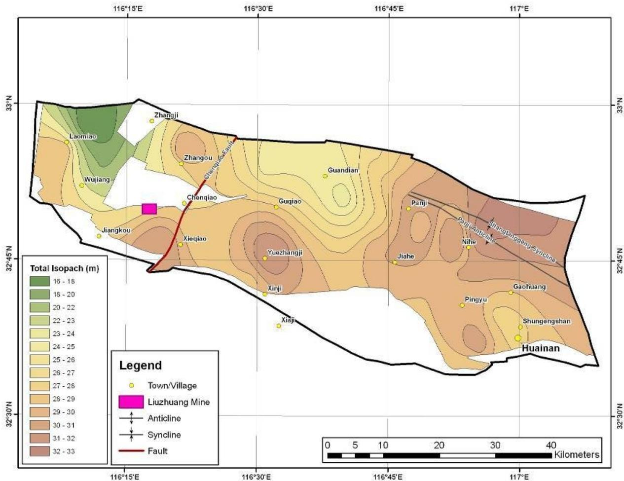
Figure 2-4: Total Coal Thickness Distribution in the Huainan Coal Field
