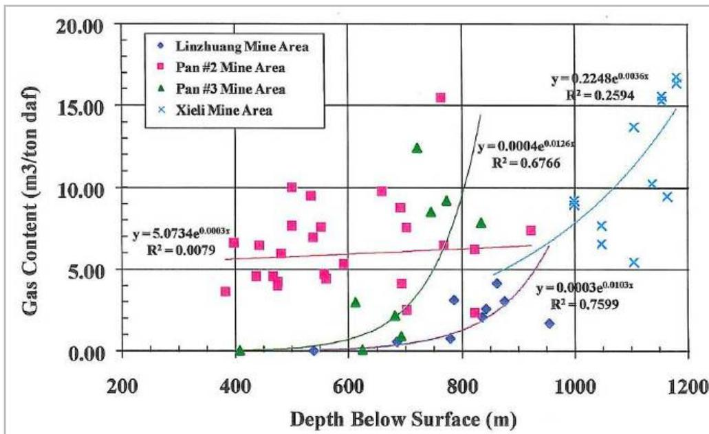
Figure 2-6: Gas Content Versus Depth in the Huainan Coal Field
