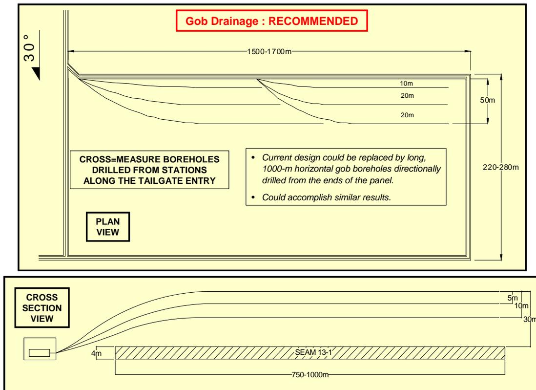
**Figure 6-7: Proposed Preliminary Engineering Design for Gob Borehole Drilling**
