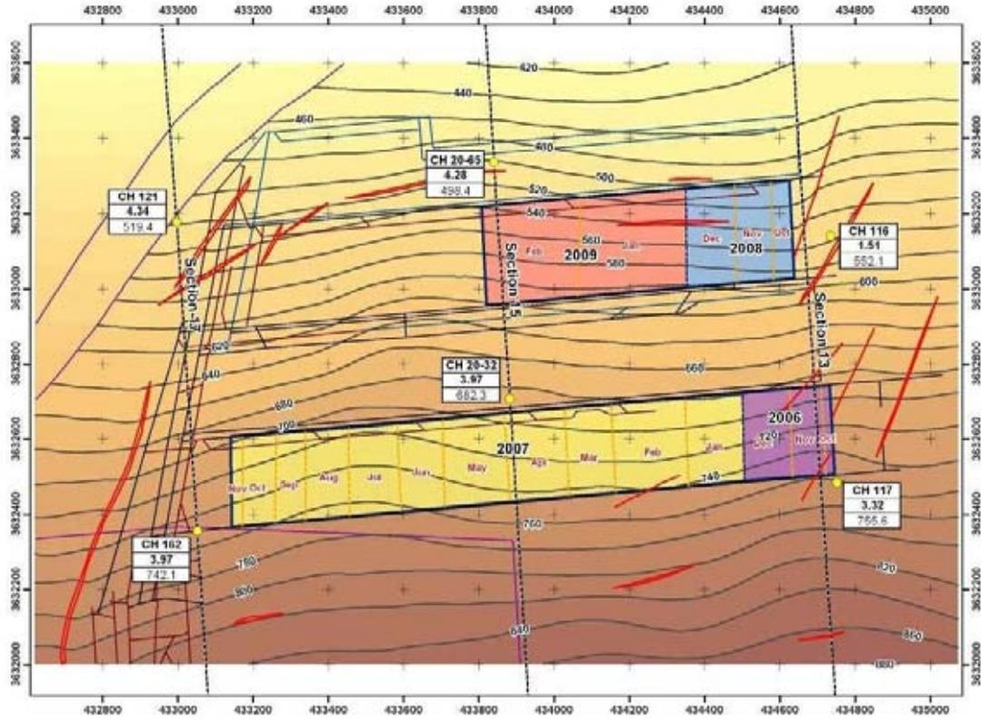
Figure 2-12: Structure and Depth to Seam 13-1 at Liuzhuang mine
