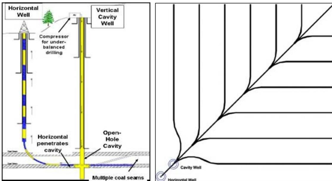
**Figure 4-21: Horizontal Pinnate Well Schematic**
