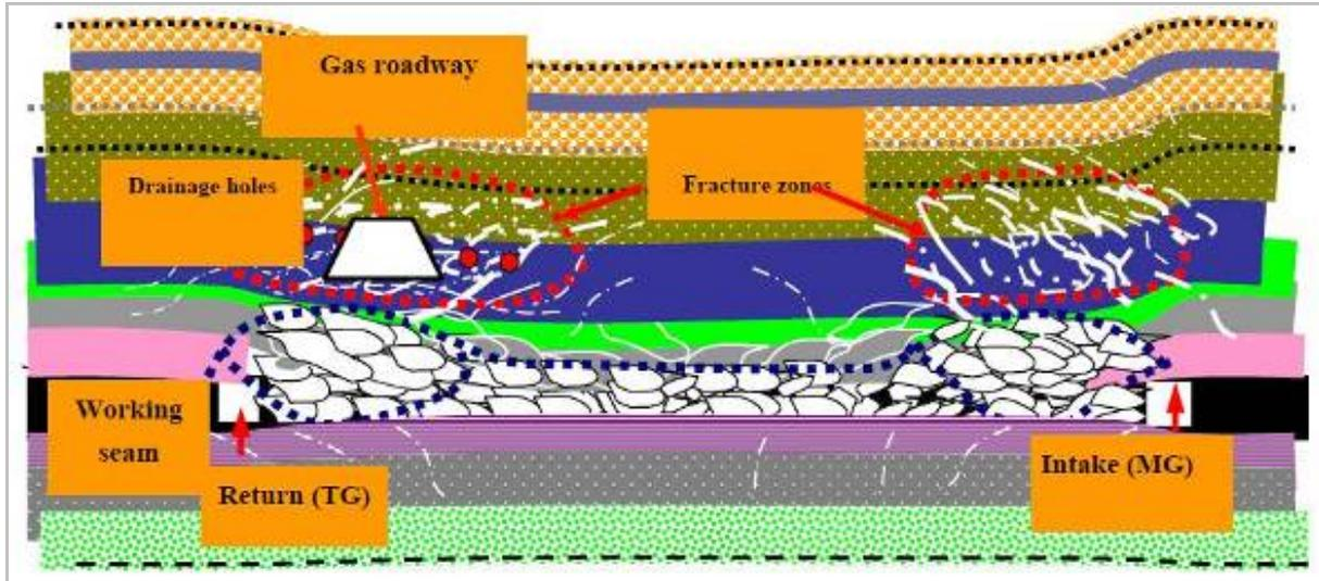
Figure 4-2: Cross-Section Typical of Liuzhuang and Other Mines in the Huainan Coal Field
