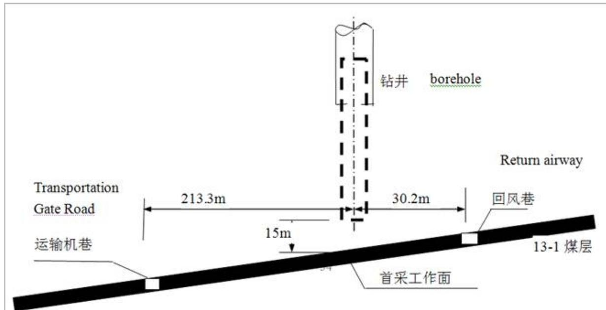
**Figure 4-24: Surface to Horizontal Gob Borehole**
