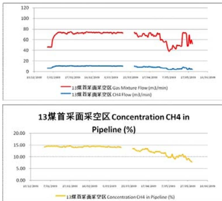
**Figure 4-7: Detailed Hourly Methane Flow Rate and Concentration**
