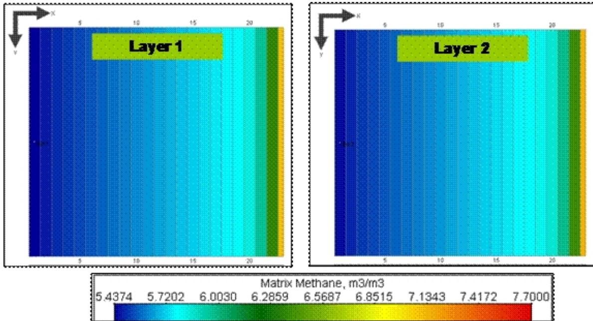
**Figure 4-19: Scenario 2 – Simulated Reduction in Gas Content**
