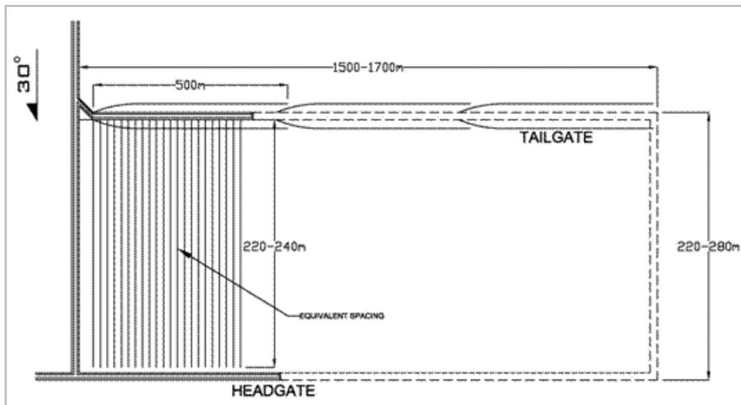
**Figure 6-2: Preliminary Engineering Design for In-Seam Directional Drilling**
