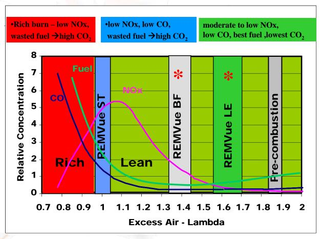
In stoichiometric or rich burn engines, much of the energy goes "up the stack" or to the catalytic converter in the form of CO and unburned methane
