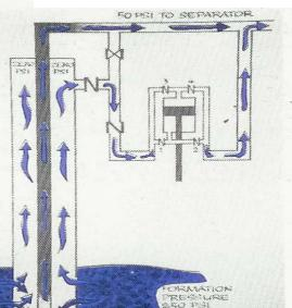
Back pressure is relieved from the face of the formation allowing more hydrocarbons to flow into the well bore.
