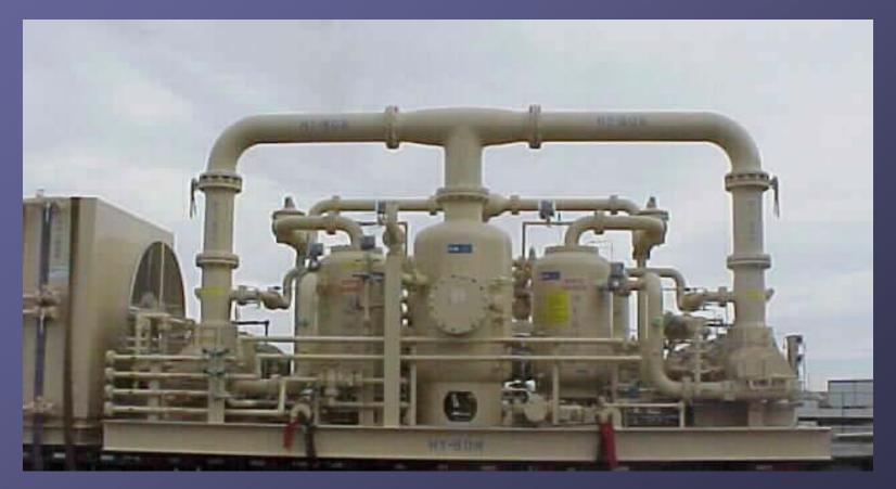
This dual flooded screw package for PDVSA is designed for volumes to 5.0 MMSCFD; moving tank vapors from 0 to 200 psig in Eastern Venezuela.
