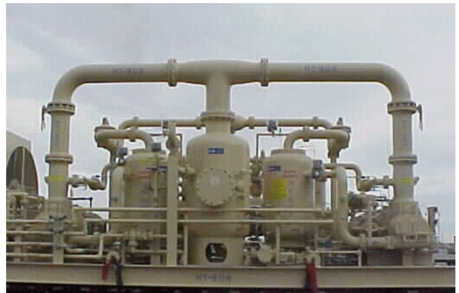
Dual VRU bound for Venezuela - one of 17 units capturing gas currently for Petroleos de Venezuela. Flooded screw compressor for volumes to 5.0 million cubic feet per day; up to 200 pounds per square inch, gauge (psig).
