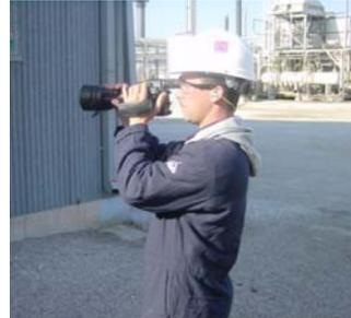
Infrared Leak Imaging Camera
