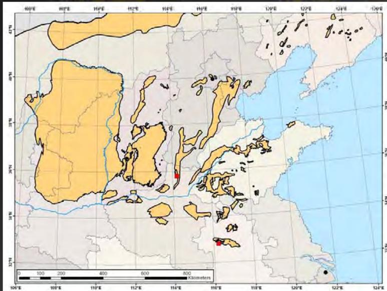
Liuzhuang is located in East China Coal Region. Faulting and fragile coals with low permeability makes in-seam drilling less effective.
