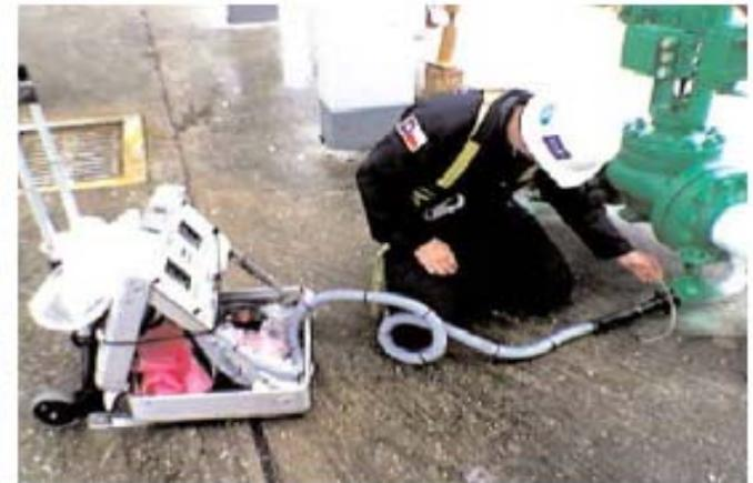
*Leak Detection and Measurement at PEMEX*
