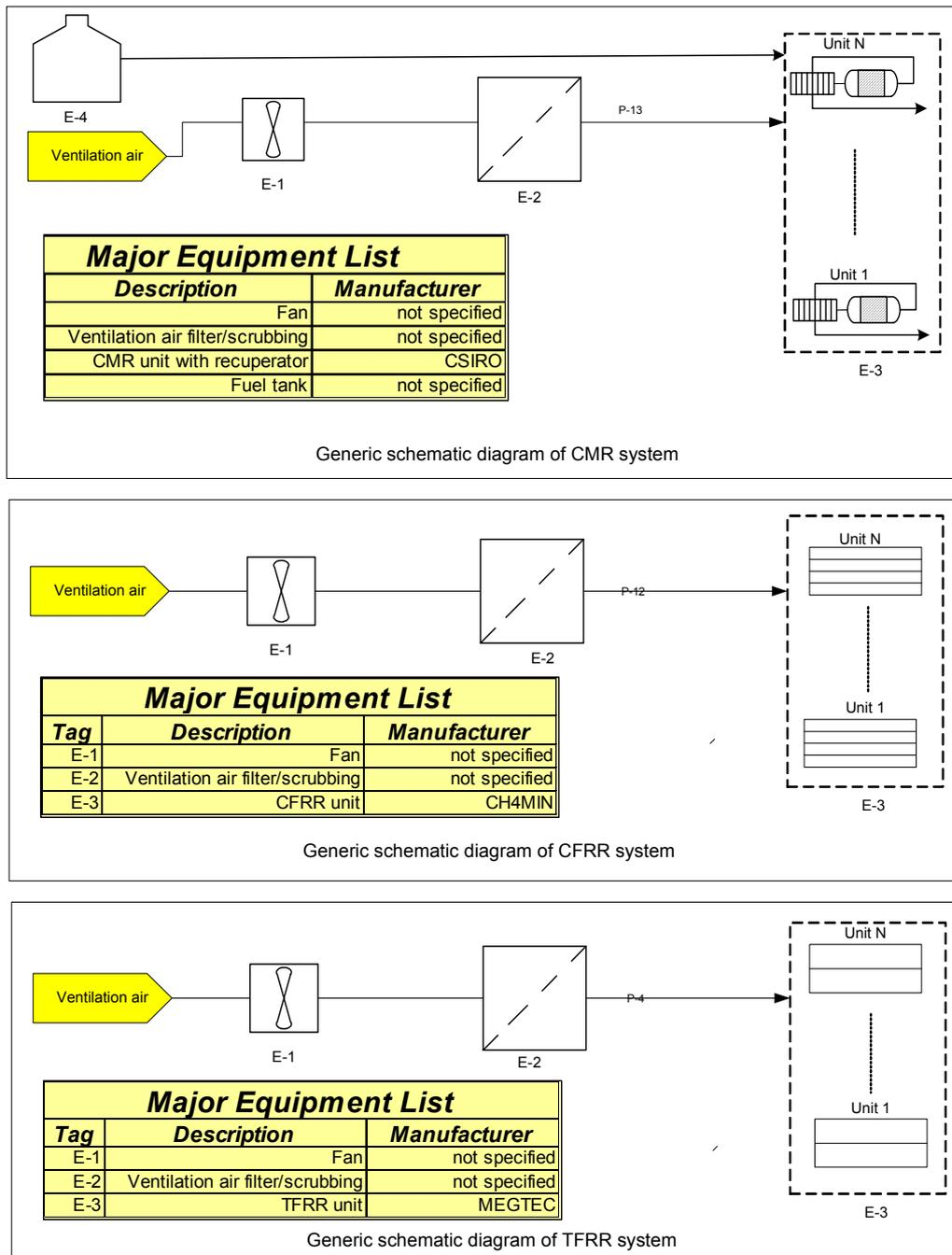
Figure 9 Configuration diagrams of TFRR, CFRR or CMR VAM mitigation plant systems
