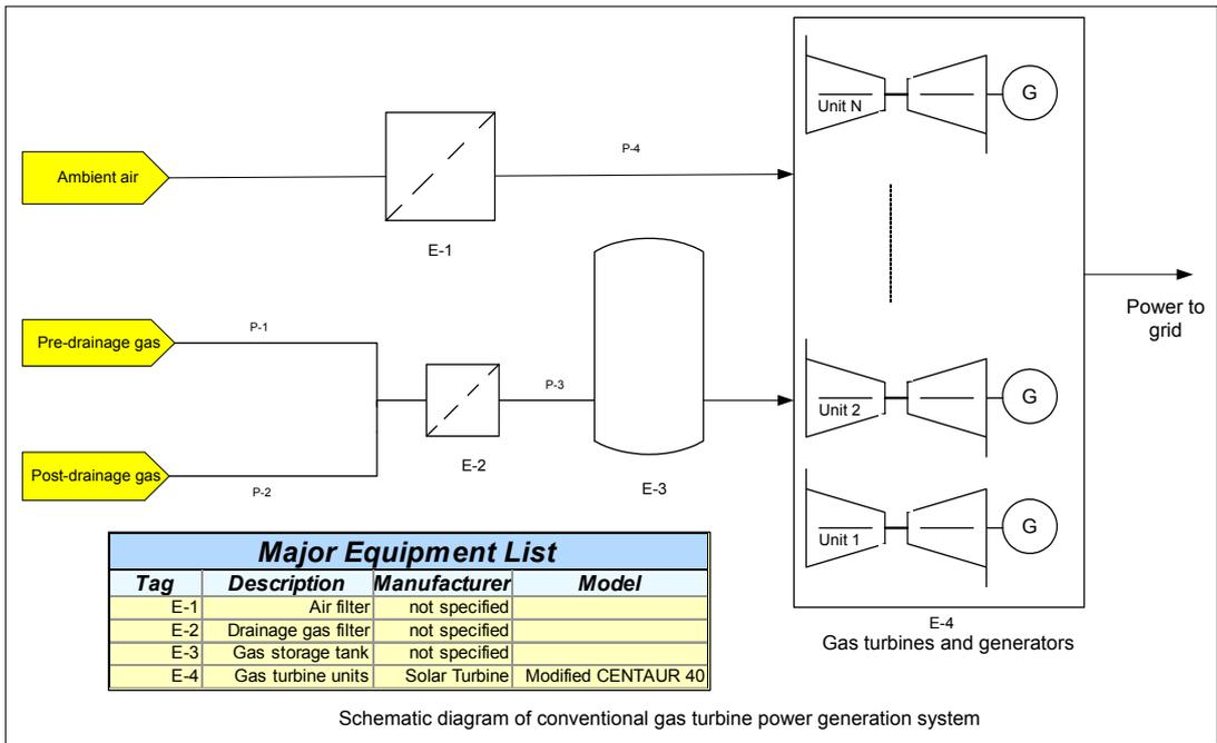
**Figure 11 Configuration diagram of drainage gas fired turbine power plant system**
