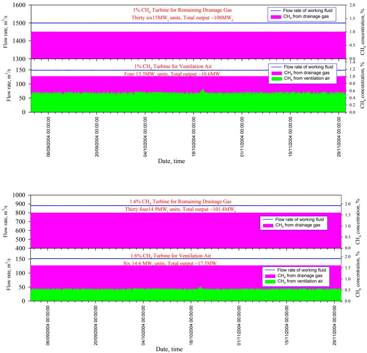
**Figure 17 Operating status of the 1% methane turbine plant at the Chinese mine**
