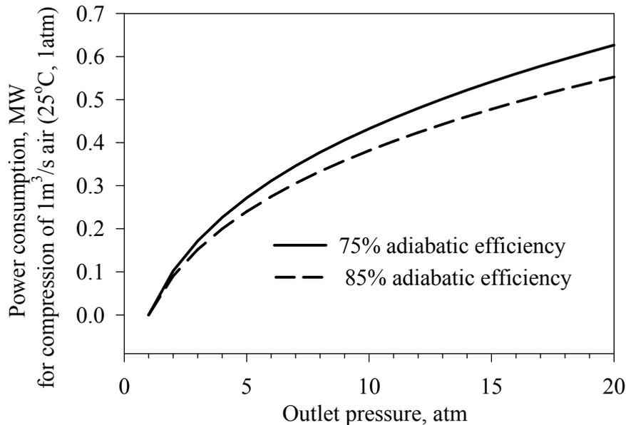
**Figure 7 Power consumption for air compression**
