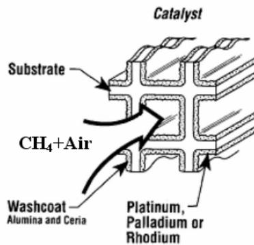
**Figure 6 Illustration of a monolith reactor [12]**
