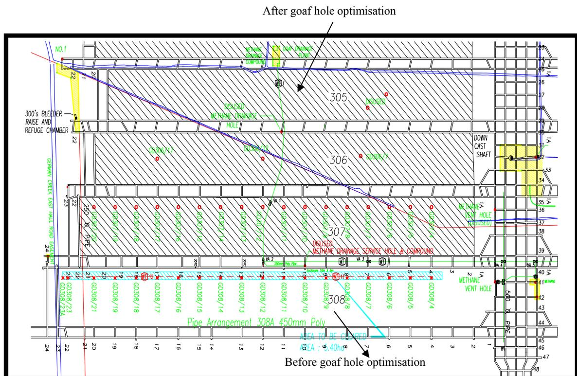
**Figure 4 Goaf drainage patterns in Mine B – before and after goaf hole optimisation [4]**
