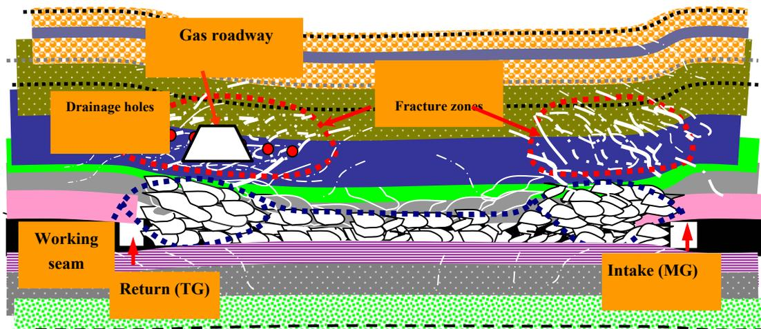
**Figure 2 Schematic layout of roof drainage borehole /gas roadway in the roof – gas drainage method in P1 mine, Huainan area [3]**
