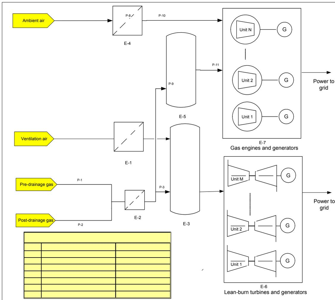
**Figure 13 Configuration diagram of the combined lean burn turbine and gas engine power plant system**
