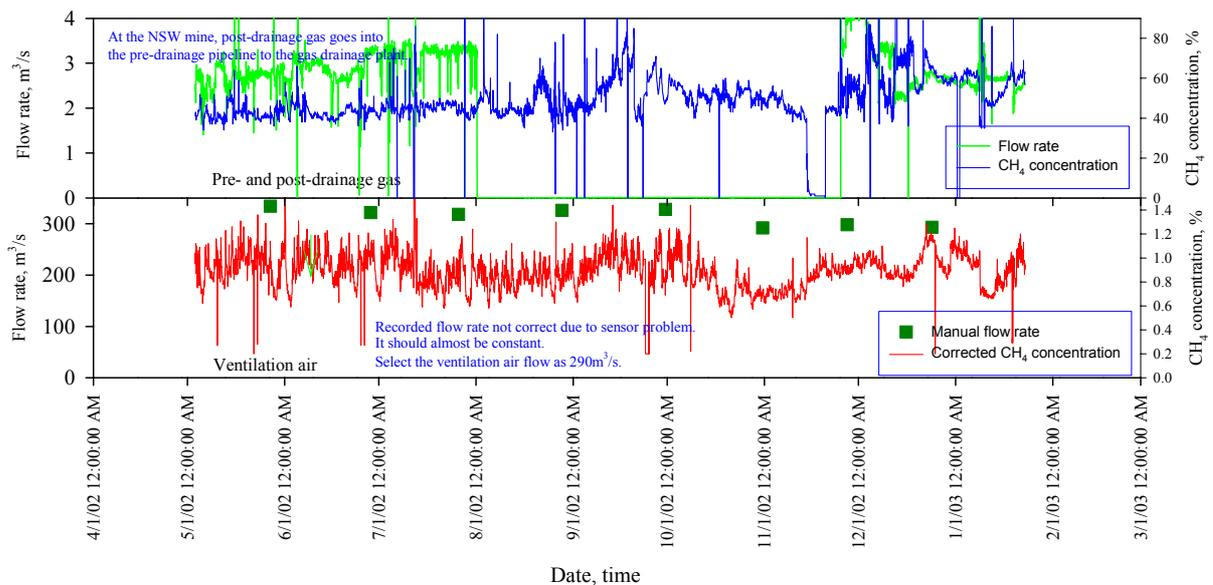
**Figure 20 Characteristics of methane emissions from the NSW coal mine**
