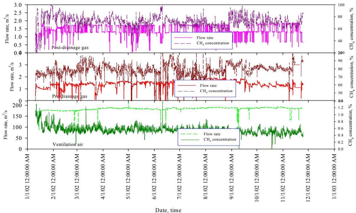
**Figure 18 Characteristics of methane emissions from a Queensland mine**
