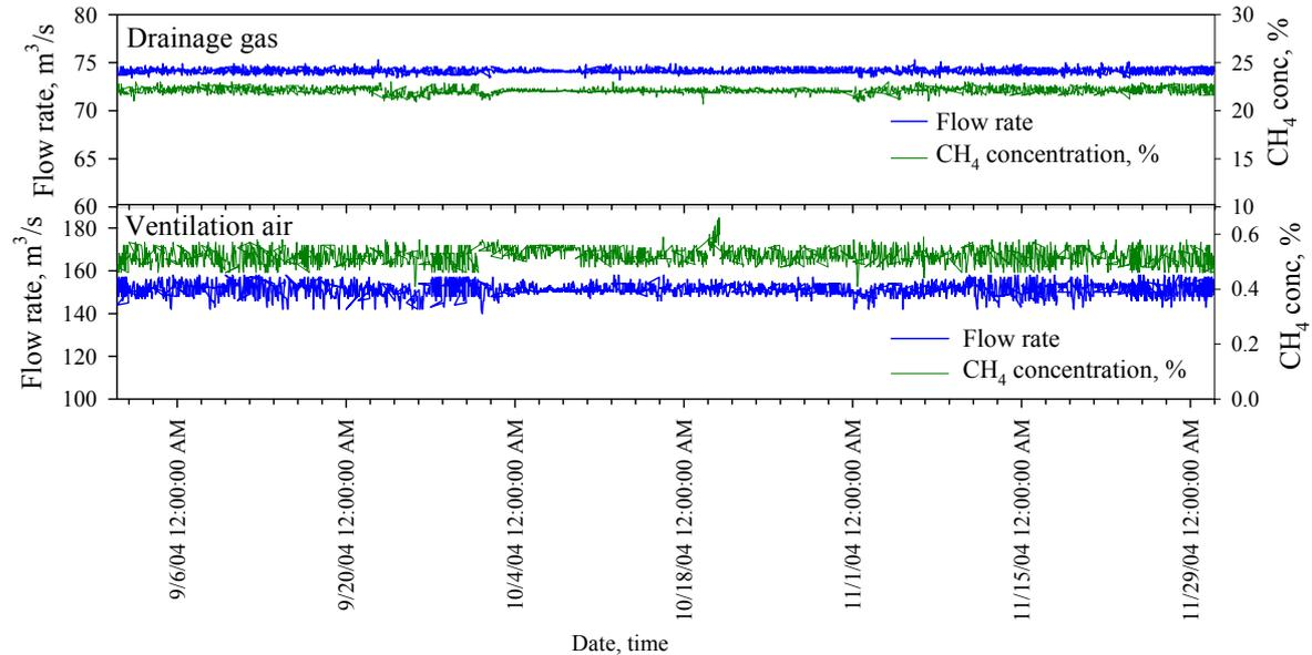
**Figure 8 Characteristics of methane emissions from a Chinese mine**
