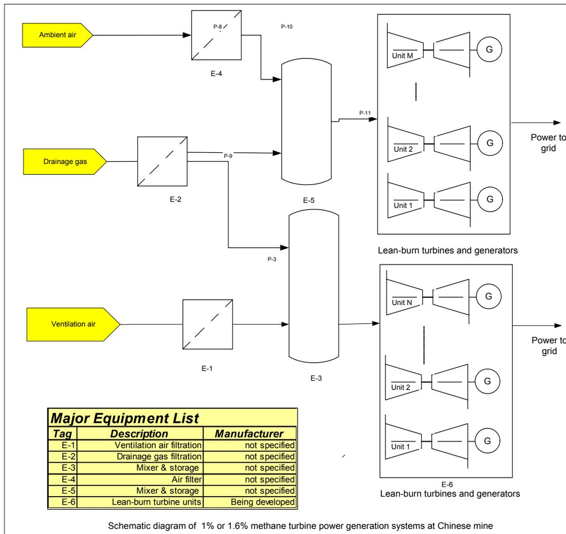
**Figure 16 Configuration diagram of the lean burn turbine power plant system**
