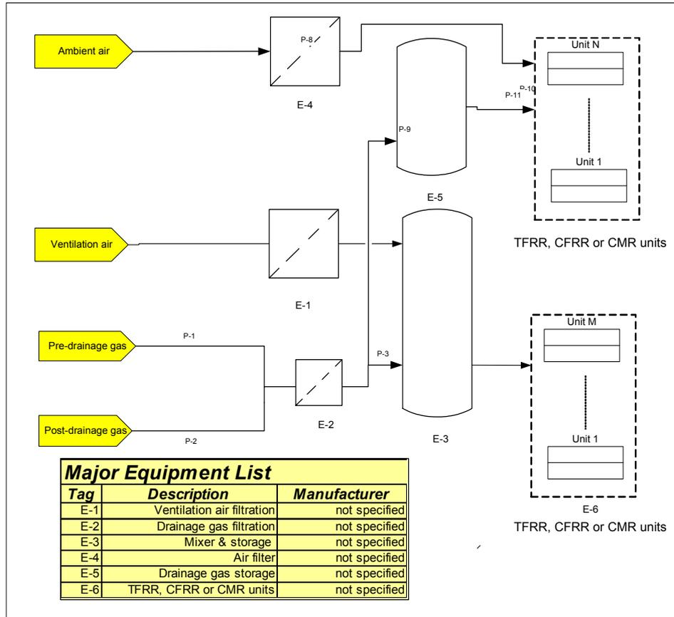
**Figure 14 Configuration diagram of the TFRR, CFRR or CMR methane mitigation plant system at Chinese coal mine**
