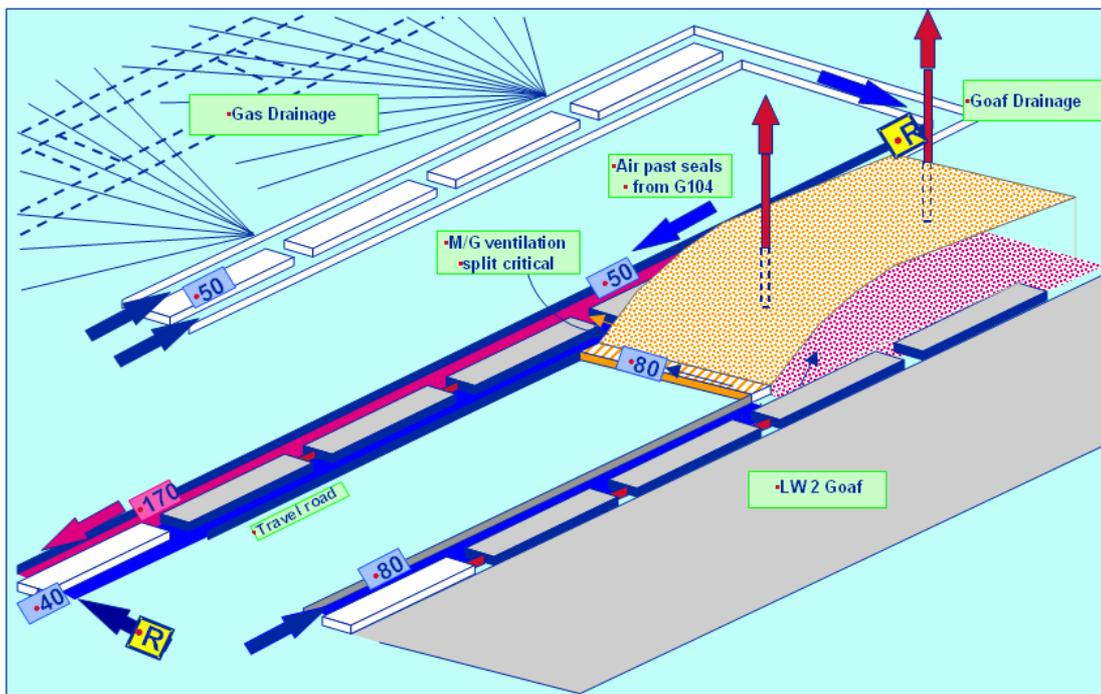
**Figure 3 Gas drainage techniques used in a typical Australian underground coal mine**
