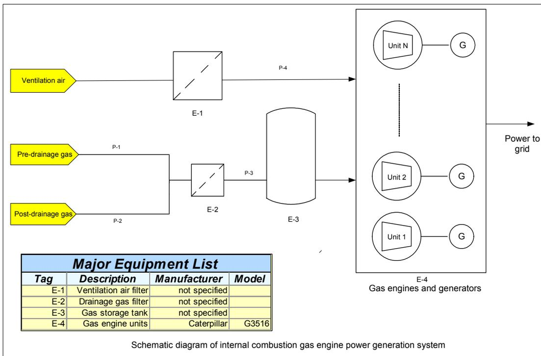
**Figure 12 Configuration diagram of drainage gas engine power plant system**
