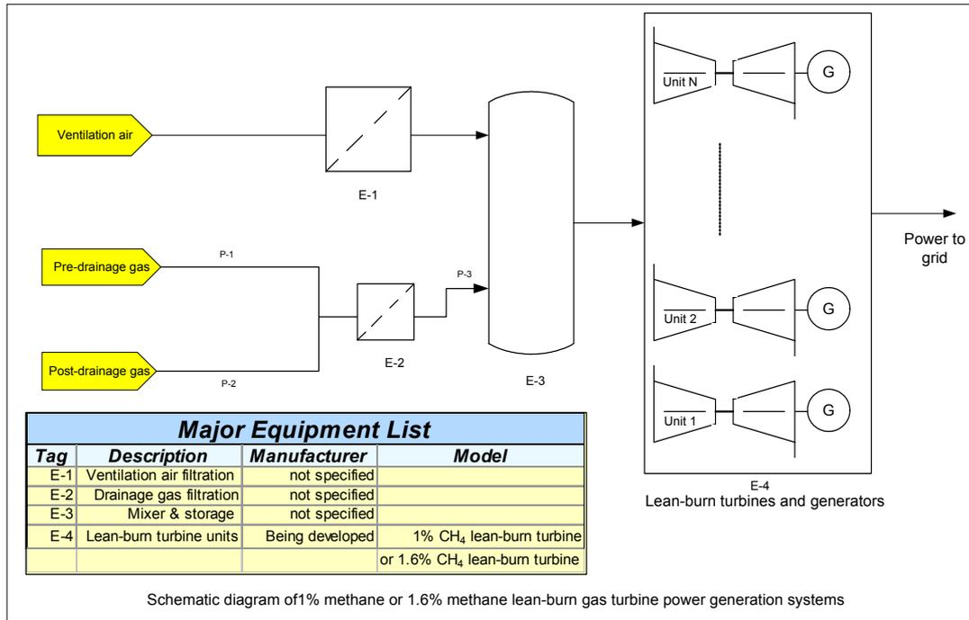
Figure 10 Configuration diagram of VAM utilisation lean burn turbine power plant system
