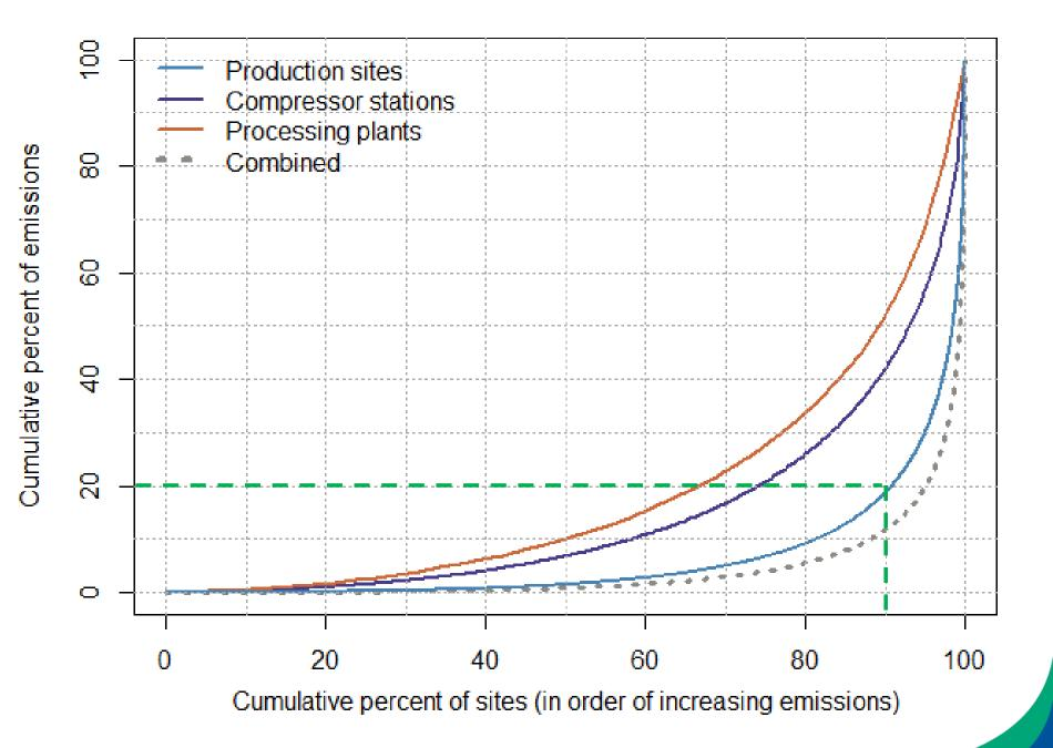
Tank flashing and liquids unloading explain the magnitude but not the prevalence of high-emitting well pads
