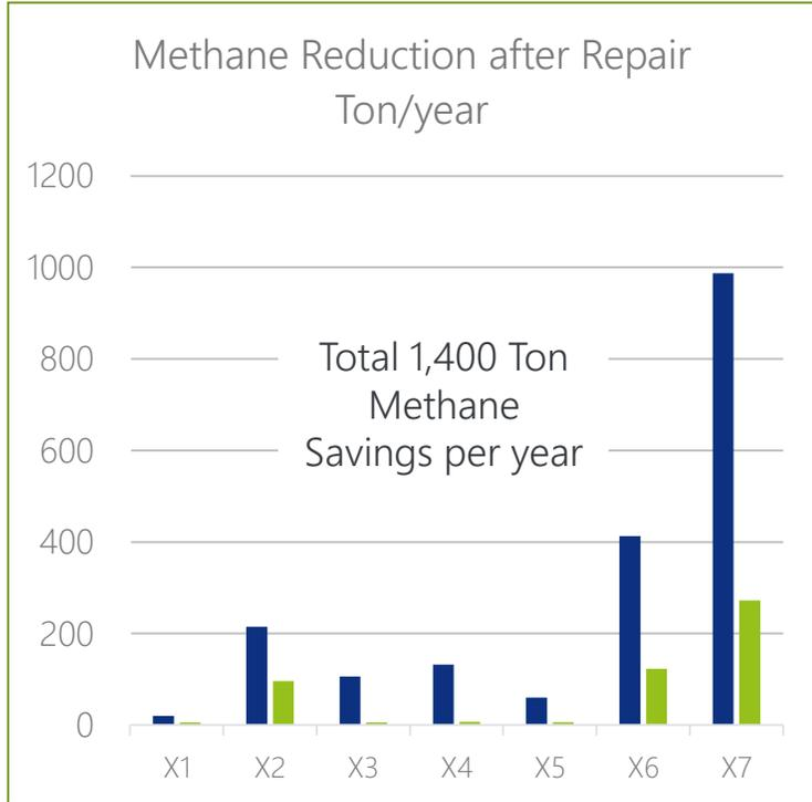
Methane Emission Reduction Results in one-year, average figures per Gas Asset type, 400 LDAR campaigns, 10mio measurements. From 1,42kg/year/source to 0,92kg/year/source or -35%
