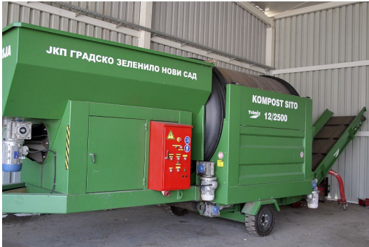
Roto sieve / 4 m3/h capacity
