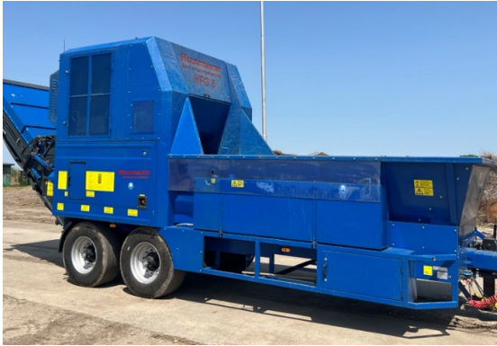
Grinder / 150-200 m3/h capacity
