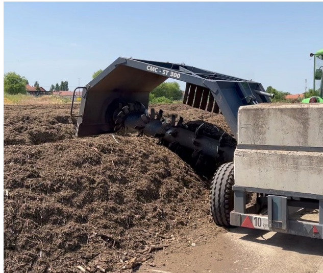
Attached compost turner / 1000 m3/h capacity
