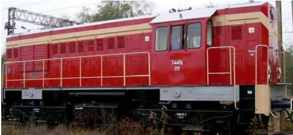
Figure 30. T448 P diesel locomotive to be adopted to fuelling with LNG
