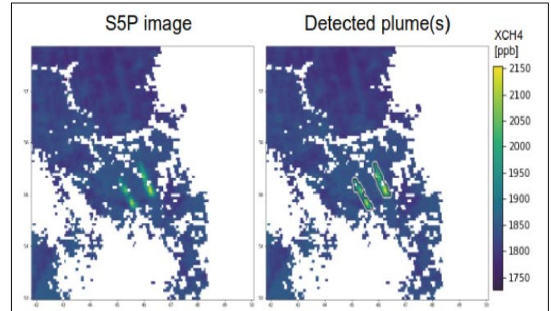
Example of high methane emission point screening based on TROPOMI data
