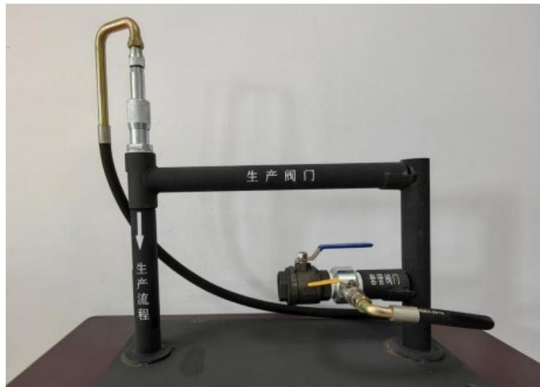
Direct-reading anti-frozen blockage constant pressure recovery valve
