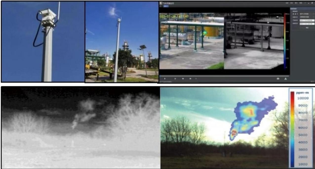
Methane Leakage Gas Cloud Imaging Monitoring System
