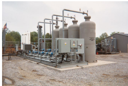
Gas Conditioning & Upgrading System for Gas Pipeline Sales Abandoned Mine, Illinois, USA
