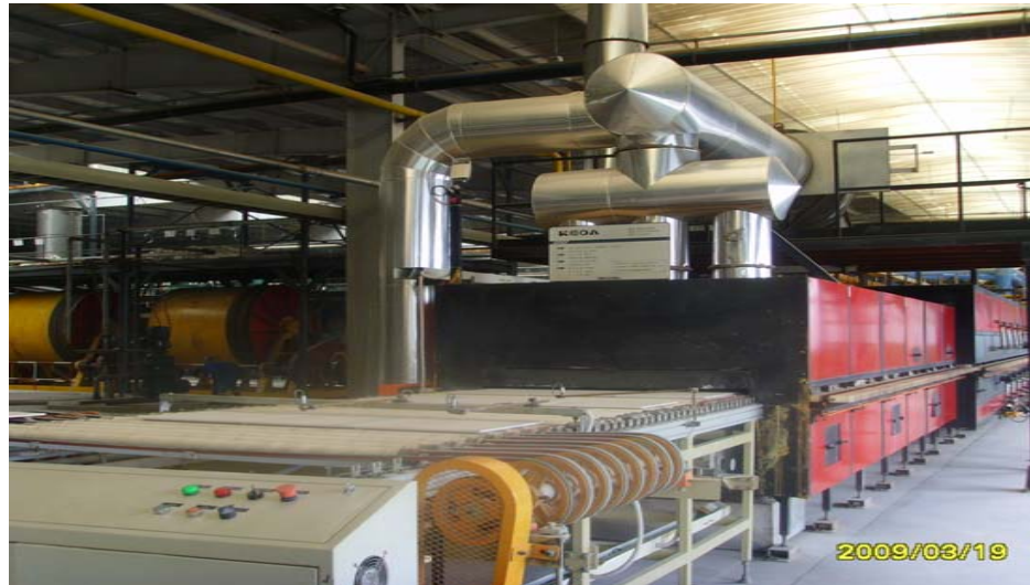
Production line of ceramic tile utilized CMM as industrial fuel
