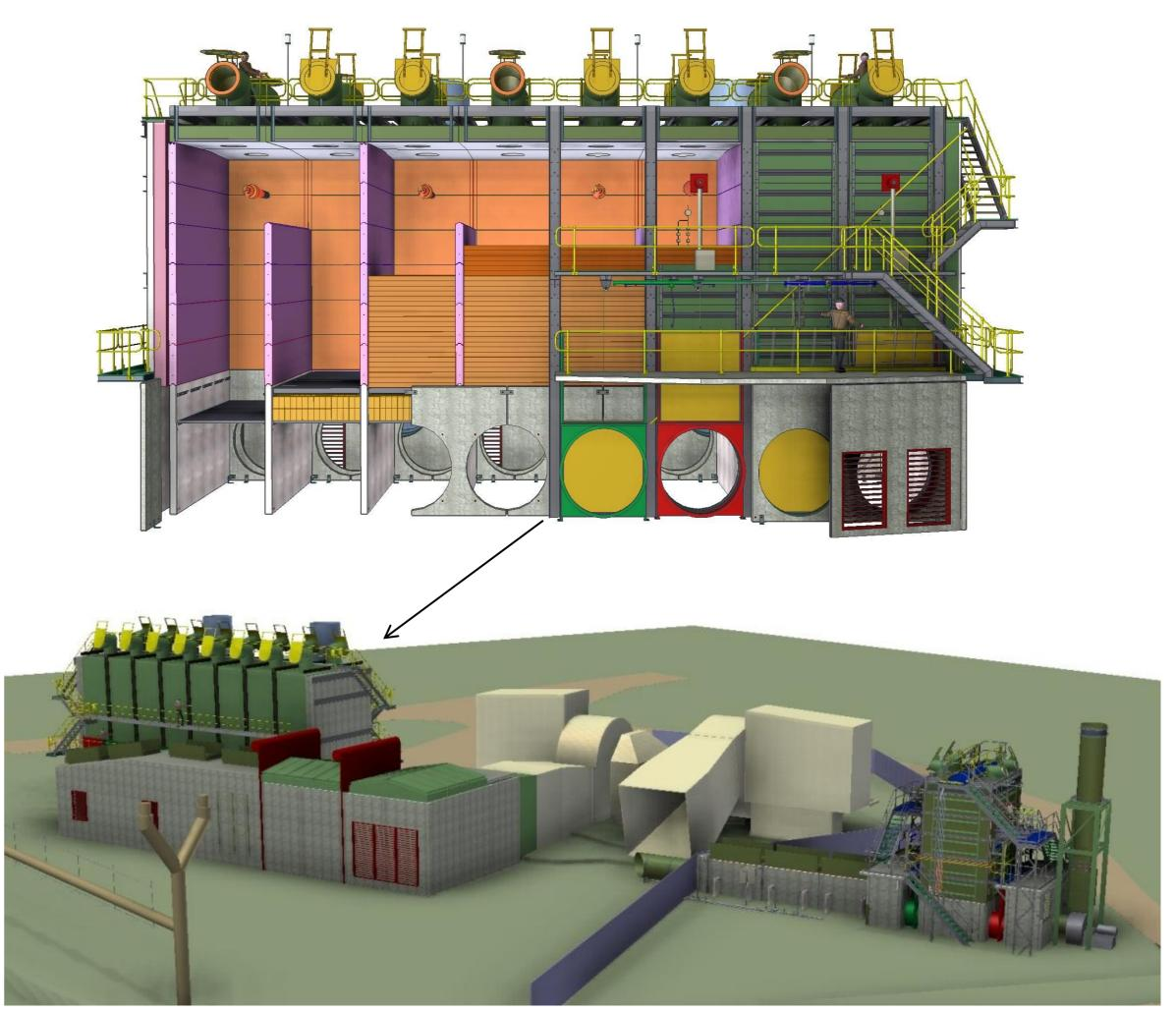
SECTION CUT-OUT OF THE COMMERCIAL SCALE 'FOUR PACK' VAM RAB
