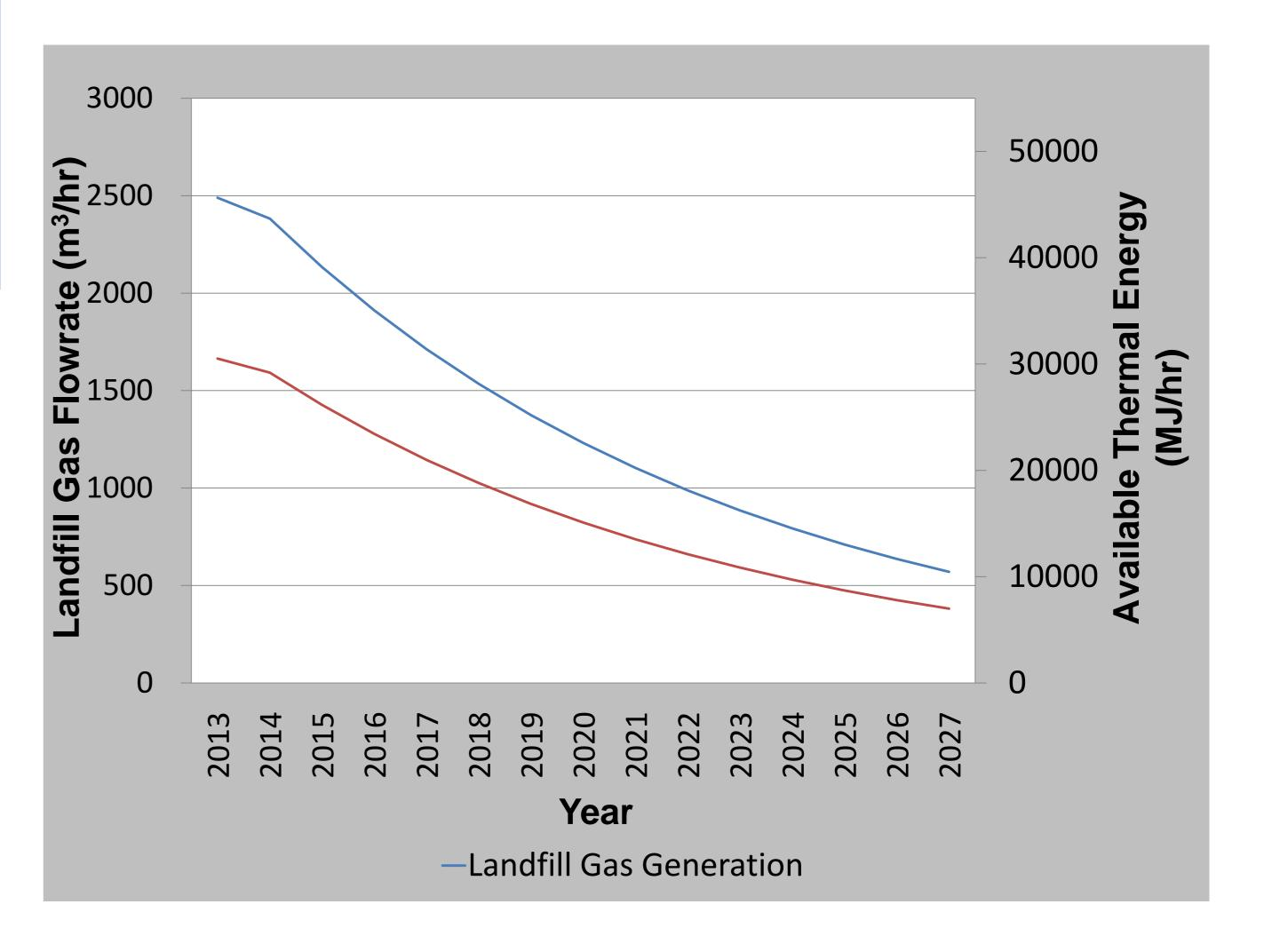
Recoverable Biogas = 50% Landfill Area Available for Gas Collection x 65% Gas Collection Efficiency = 33%
