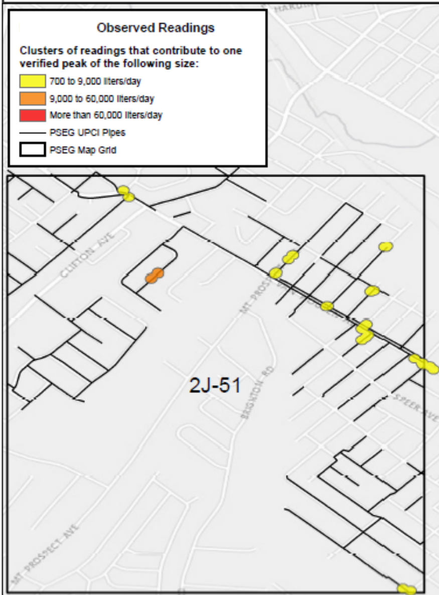
Overlap of Pipes and Observed Data from EDF Methane Mapping
