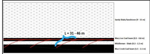
Borehole Placement from Adjacent Drillable Horizons
