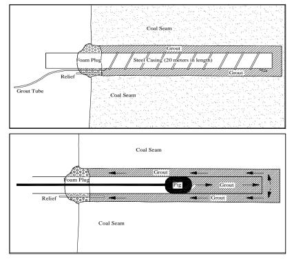
Initial and Secondary Grouting with Pressure Testing
