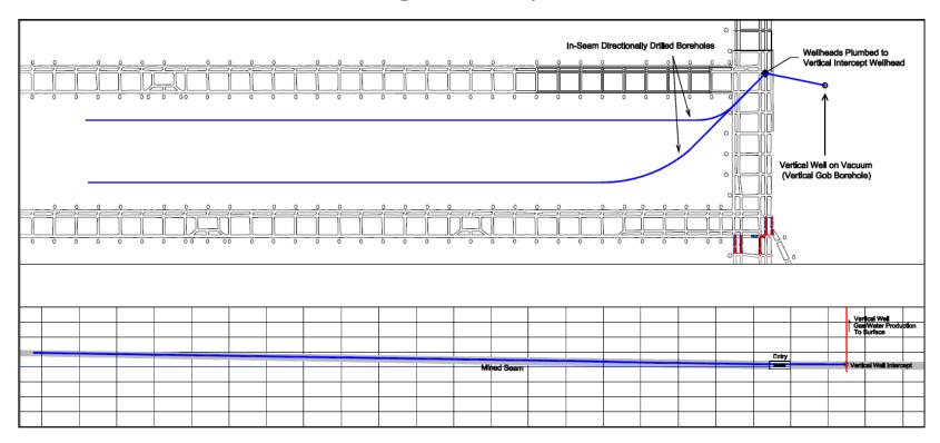
Gas Production Moved to Surface via Interception with Nearby Vertical Well or VGW with water separation in entry
