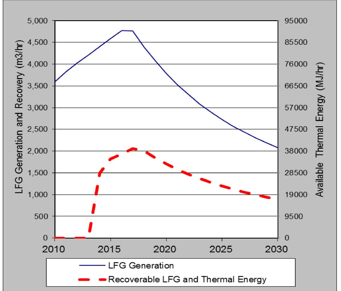
Values for these modeling variables have been developed based on the waste composition data and average annual precipitation at the Vinca Landfill. It is not feasible to collect all the gas generated at the site for flaring or energy recovery given site conditions and collection system limitations. Therefore, the amount of recoverable LFG was estimated by applying a gas availability factor to the results of the LFG generation model (graph above).
