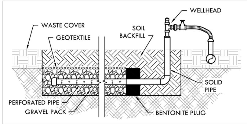
**Figure 3-2. Horizontal Extraction Well**
