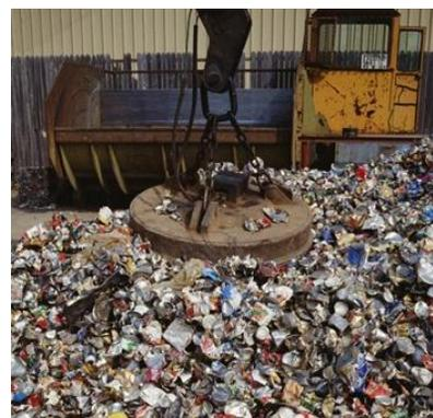
**Figure 1-5. Metal Sorting at Materials Recovery Facility**
