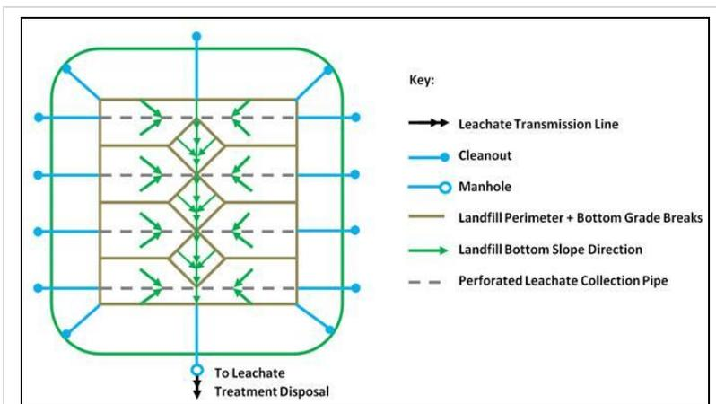
Figure 2-1. Typical Layout of Leachate Collection System (top view)
