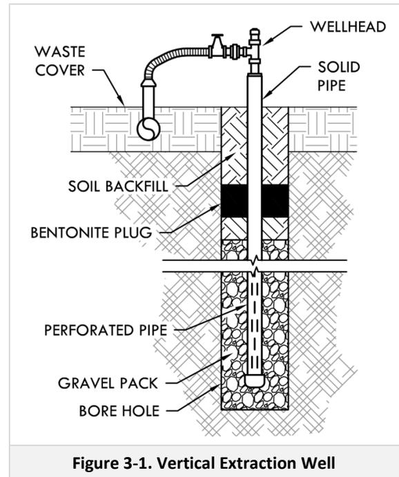
Figure 3-1. Vertical Extraction Well
