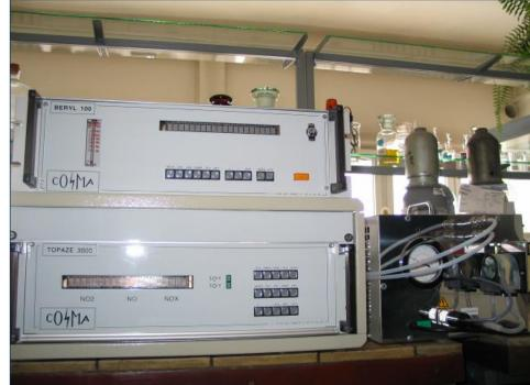
a TOPAZ 3020 analyser for continuous testing NO/NO<sub>X</sub>/NO<sub>2</sub>, a BERYL 100 analyser for continuous testing CO.
