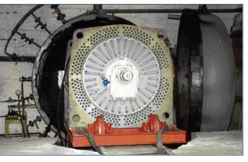
The chamber for testing explosion propagation
