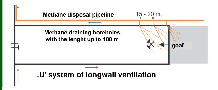
Efficiency of methane drainage – 20% ÷ 40%
