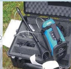
Volumetric emissions measuring and detection device
