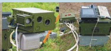
Board passive distant gas meter for methane concentration "Tomsk-1"
