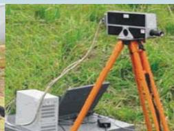
DGA of methane concentration based on an IrDA sound and optical spectrometer and projector
