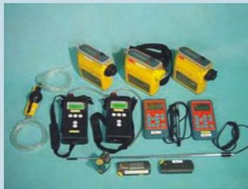
Leakage detectors, methane concentration meters
