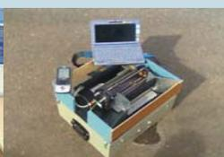
Laser measuring system of the methane local concentration
