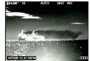
VOC emissions visible during lightering operations.
