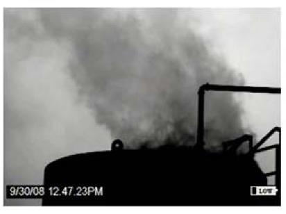
Vented emissions are not readily visible or identifiable without specialized equipment yet they represent significant natural gas losses, reduced operational efficiency, greenhouse gas emissions and potential safety risks.
