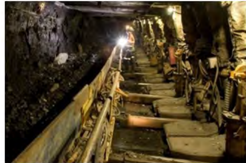
An active longwall mining operation
