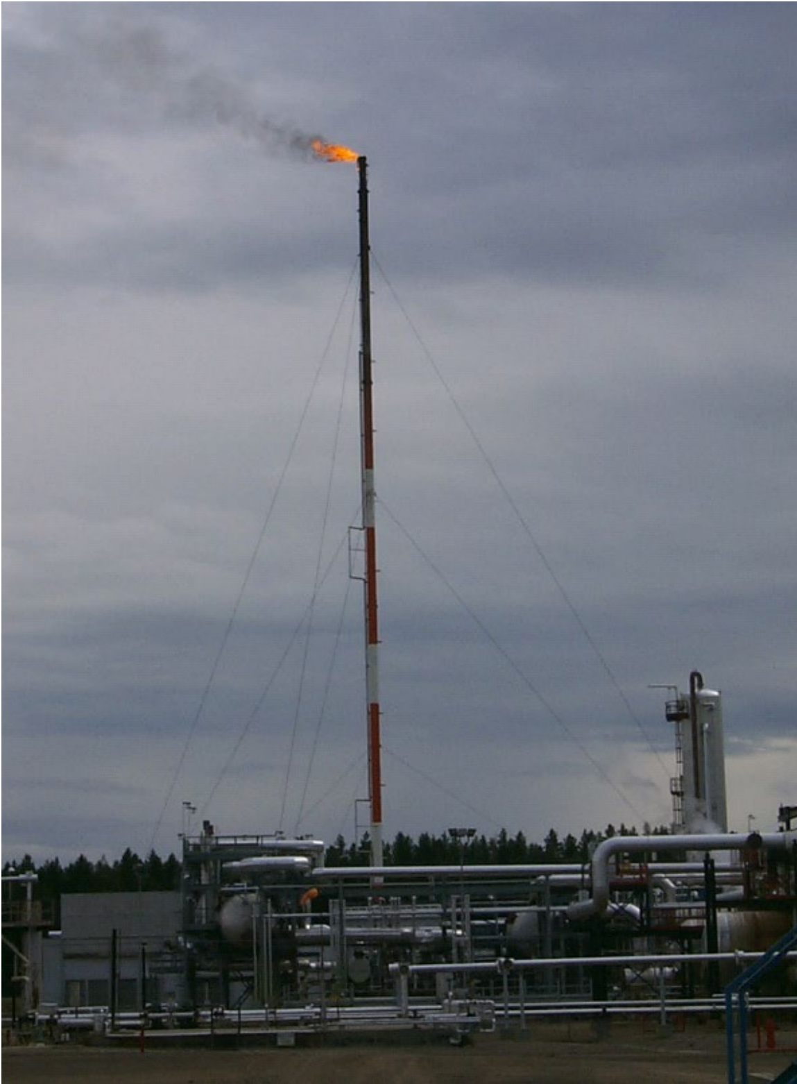
Figure 9: Photograph of a typical flare at an upstream oil and gas facility
